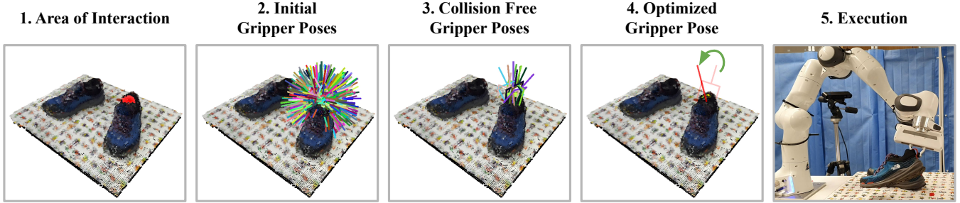
Fig. 3. Manipulation module \mathcal{O}_T : Given the proposed area of interaction \mathcal{A} , random gripper poses are initialised at each coordinate \mathbf{x} \in \mathcal{A} . Then, collision-free poses are retained and optimized, using Eq. 5. The gripper pose with the lowest final loss score is then sent to the motion planner.
